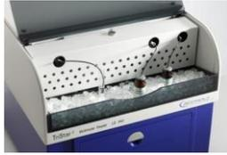
\*\* The instrument can have up to 3 internal bellows type reagent **"JET" injectors**. All of the injectors are in the front of the instrument for easy access and can be chilled on ice with our waterproof tray. Two of the injectors are in the Luminescence measurement position for true flash assays and the other is in the pre-measurement position from 10ul to 100ul volume and can be used with 384 well applications.
