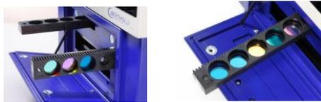
\*\* The instrument also has a 5-position **emission filter slide** and 5-position **excitation filter slide**.
